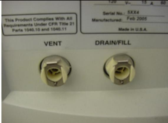
In the back of the Laser there are two white fittings labeled “VENT” and “DRAIN/FILL”. They are underneath the serial number and to the left of the power cable. With your laser you received a “Fill Funnel Kit” that consists of two hoses with white fittings on one end. One is blue and it has a yellow funnel at the other end, and the other one is black.
