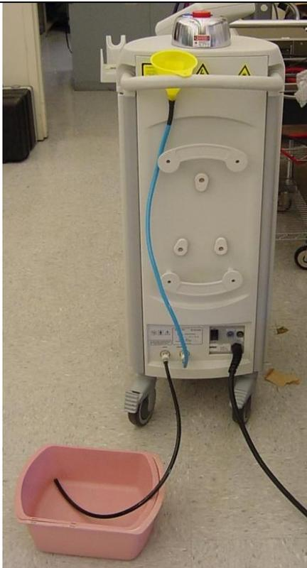
Connect the Blue hose first. Keep it high to prevent draining water out. The best way to do that is to thread the hose between the handle and the console, to support the funnel at the proper level. Plug the other end of the hose to the right fitting labeled “DRAIN/FILL” (see pictures). Fill funnel with distilled water. Always keep water in the funnel to prevent air bubbles from entering the hose.
